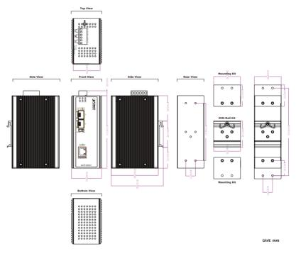
Figure 1: IGUP-1205AT Three-View Diagram
