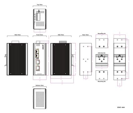
Figure 2: IGUP-2205AT Three-View Diagram
